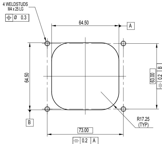
Note: Adapter plate is available to fit the new US85 to the old stud positions
