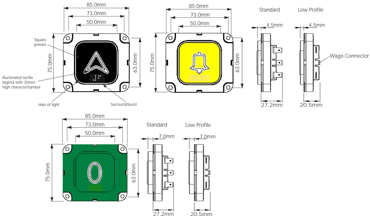
Jumbo Pushbuttons can be supplied loose or incorporated into stations with 1.5mm or 2.5mm stainless steel faceplates, with a vertical pitch of 80mm and horizontal pitch of 90mm i.e the pushbutton body can be rotated through 90 degrees (horizontal version shown above). If pushbuttons are supplied loose, spacers are provided to accommodate the differing faceplate thickness.
