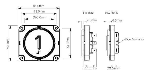
Jumbo Pushbuttons can be supplied loose or incorporated into stations with 1.5mm or 2.5mm stainless steel faceplates, with a vertical pitch of 80mm and horizontal pitch of 90mm i.e the pushbutton body can be rotated through 90 degrees (horizontal version shown above). If pushbuttons are supplied loose, spacers are provided to accommodate the differing faceplate thickness.
