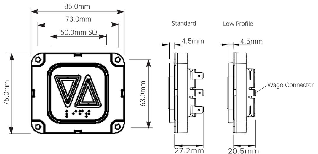
Jumbo Pushbuttons can be supplied loose or incorporated into stations with 1.5mm or 2.5mm stainless steel faceplates, with a vertical pitch of 80mm and horizontal pitch of 90mm i.e the pushbutton body can be rotated through 90 degrees (horizontal version shown above). If pushbuttons are supplied loose, spacers are provided to accommodate the differing faceplate thickness.
