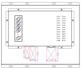
Note 4: The minimum mounting clearance required for the cable entry is indicated by the red boxes.
