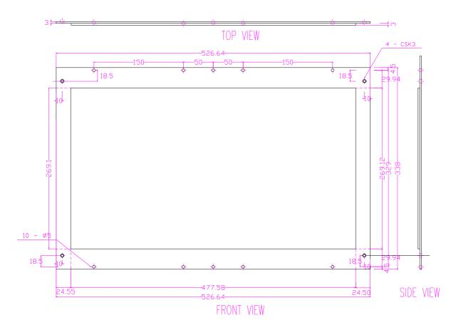
Note 1: Window cut-out is reference to Lens cut-out +0.5mm (tolerance)
