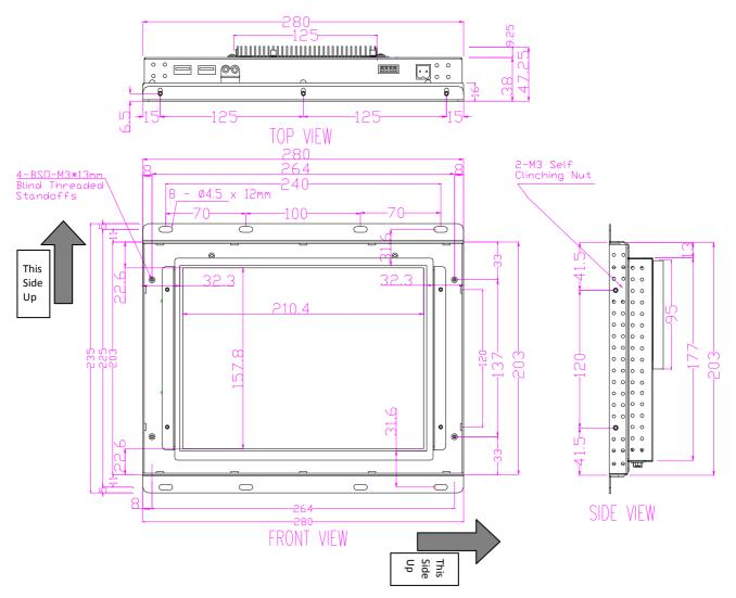
Note 1: Lens is optional item. Dimension will be provided separately. Window cut-out should reference to Lens cut-out (if any)
