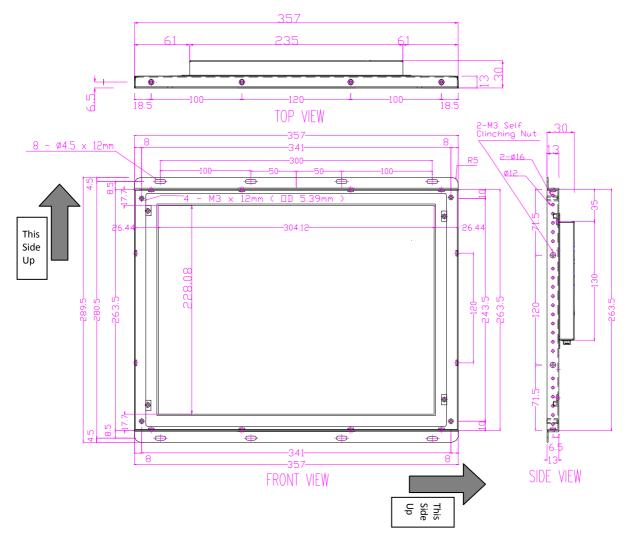
Note 1: Mounting Hole of open Frame is identical to Main Display
