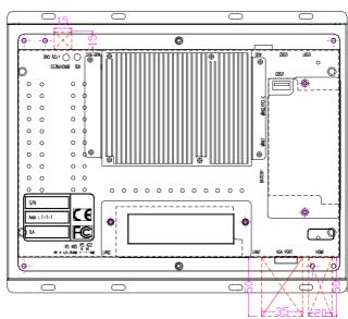
Note 3: The minimum mounting clearance required for the cable entry is indicated by the red boxes.
