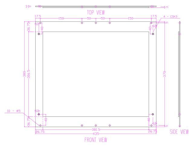
Note 1: Window cut-out is reference to Lens cut-out +0.5mm (tolerance)
