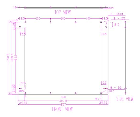
Note 1: Window cut-out is reference to Lens cut-out +0.5mm (tolerance)
