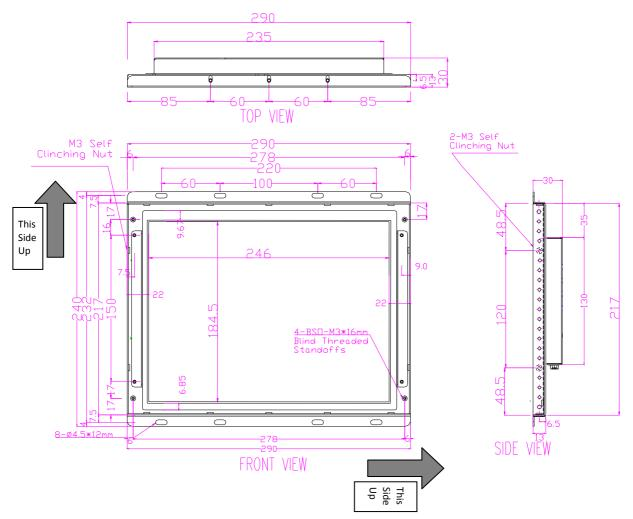
Note 1: Mounting Hole of open Frame is identical to Main Display
