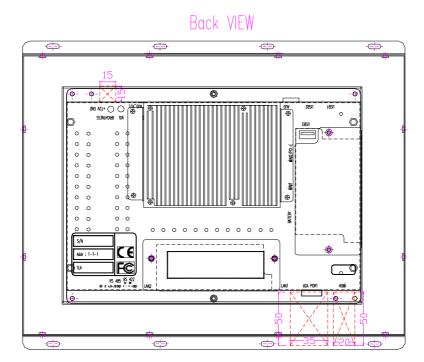
Note 3: The minimum mounting clearance required for the cable entry is indicated by the red boxes.
